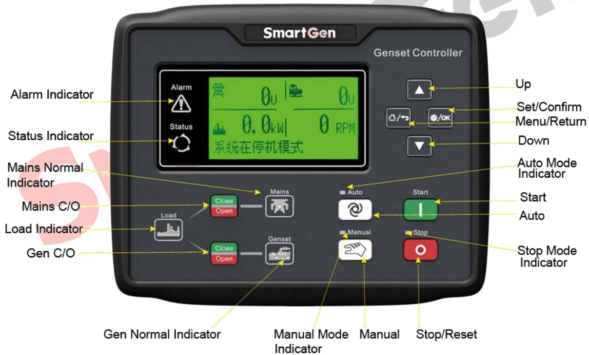
Figure 1 - HGM7110N Front Panel Indication
