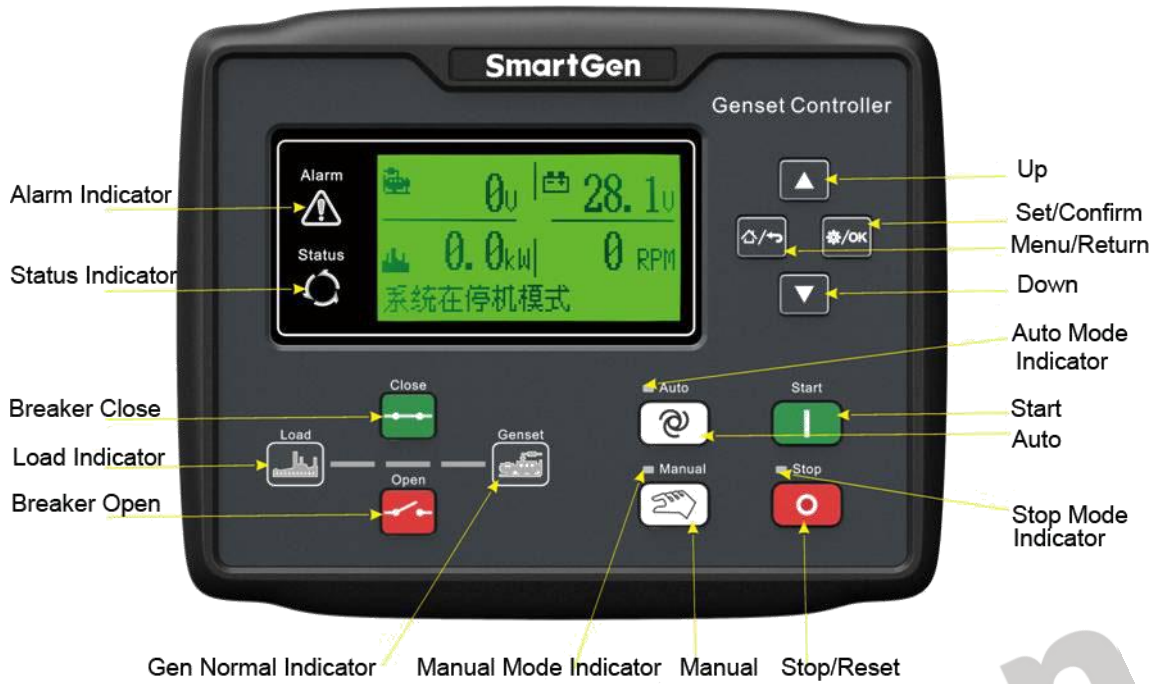
Figure 1 - HGM7110N Front Panel Indication
