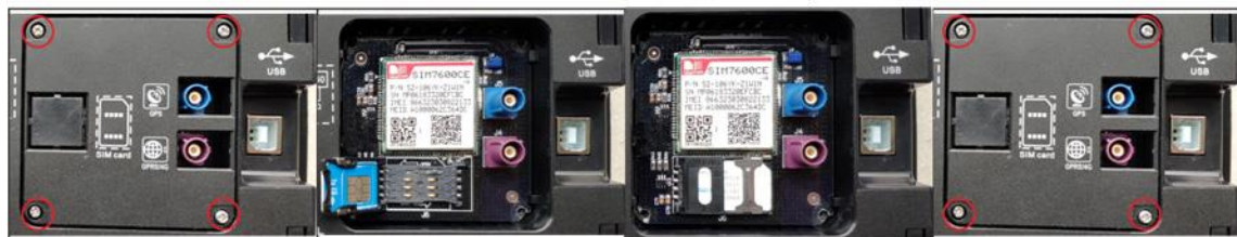
Fig.9 SIM Installation Steps
