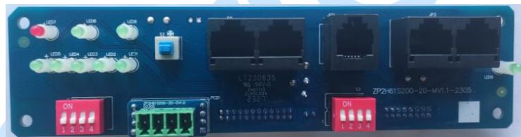
Fig.8 – HP16S100-10 Communication Board
