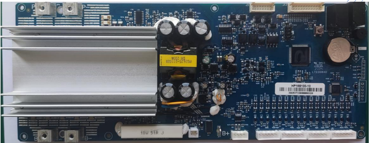
Physical Image of Lithium Battery Protection Board
