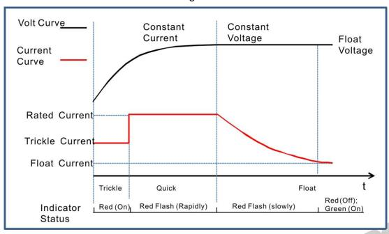
Charging is performed according to the battery charging characteristics using two-stage method.
