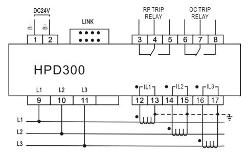
Fig.3 - 3 phase 3 wire/3 phase 4 wire
