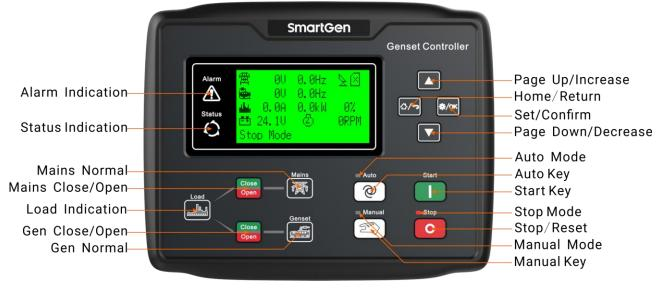
Fig.1 - HGM6120T Front Panel Indication
