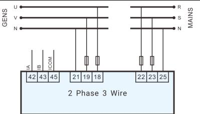
Fig.6 – 2 Phase 3 Wire Diagram
