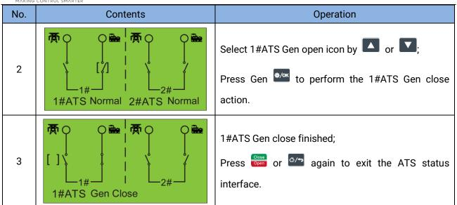
Note: When there is only 1#ATS, it will perform the corresponding switch on/off action by pressing Mains or Generation in manual mode.
