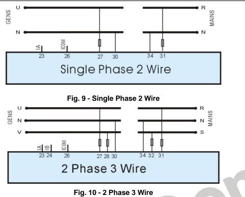
**ANote:** Recommend that the output of crank and Fuel expand high capacity relay.
