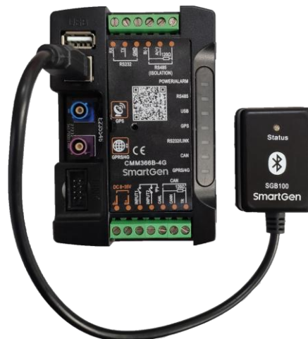
Fig.9 – USB and SGB100 Module Connection Diagram
