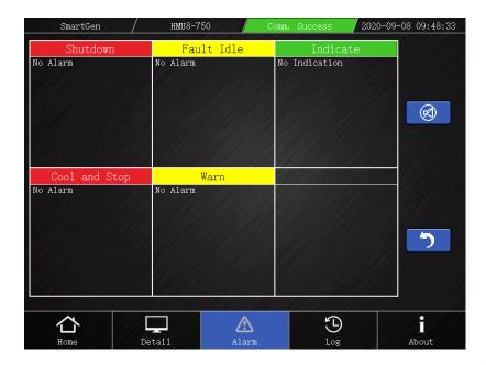
Fig.4-Alarm Display Interface
