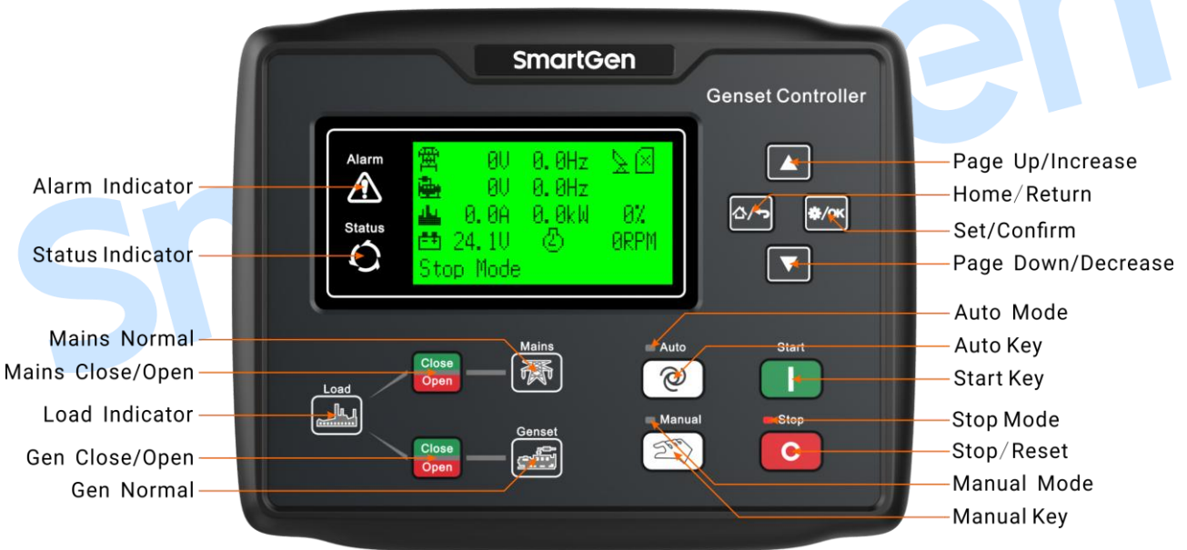
Fig.2 - HGM6120-4G(HGM6120N-4G/CAN-4G) Front Panel Indication
