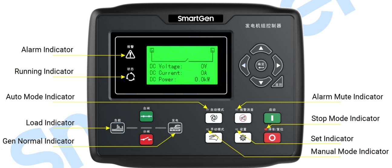
**Fig. 1 - Controller Front Panel**
