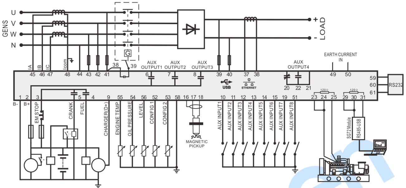
**Fig.4 - HGM8110ZDC Typical Application Diagram**
