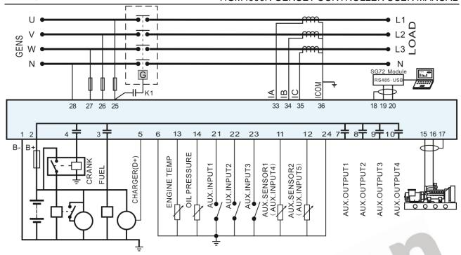
Fig.6 - HGM4010CAN Typical Application
