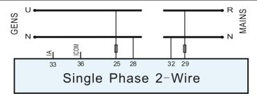
Fig.8 - Single Phase 2-Wire Connection Diagram
