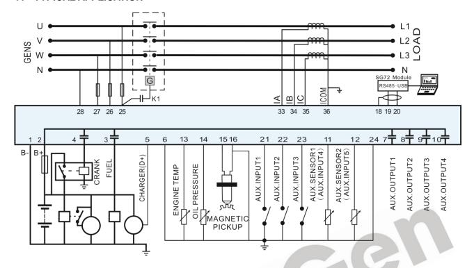
Fig.4 - HGM4010NC Typical Application
