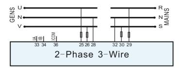
Fig.9 - 2-Phase 3-Wire Connection Diagram
