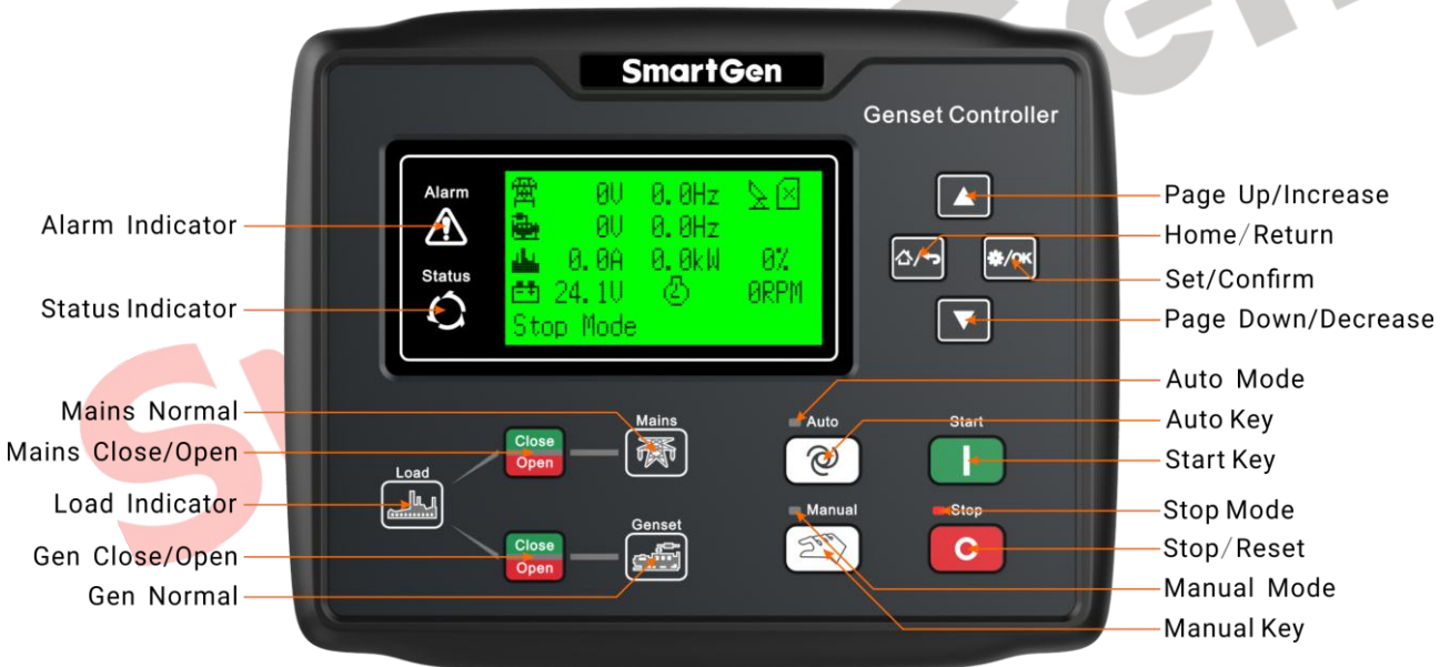
Fig.2 - HGM6120-4G(HGM6120N-4G/CAN-4G) Front Panel Indication
