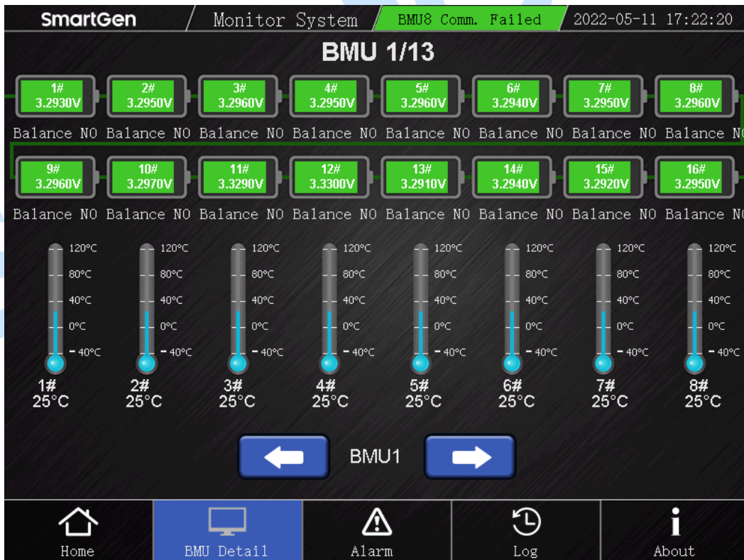
Fig.9 – Details Interface of HMU8-BMS
