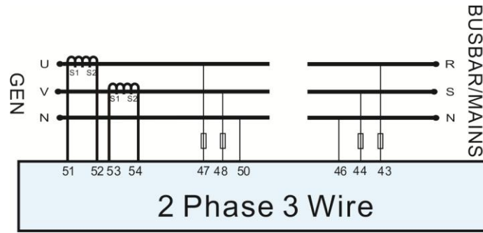
Fig. 12 2-Phase 3-Wire Application Diagram
