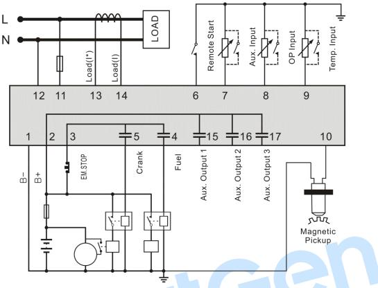
Fig.7 HGM1790N Typical Application Diagram
