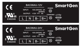
Fig. 2 BAC06AU Panel Mask
