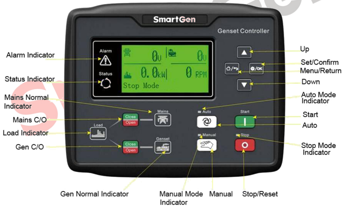
Fig. 1 - HGM7110N Front Panel Indication
