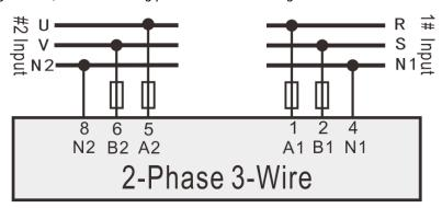
Fig. 9 - 2-phase 3-wire Wiring Diagram
