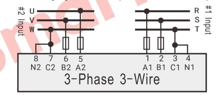
Fig. 11 – 3-phase 3-wire Wiring Diagram
