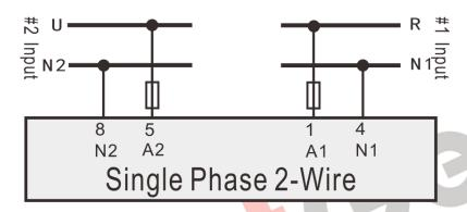
Fig. 10 - Single Phase 2-wire Wiring Diagram
