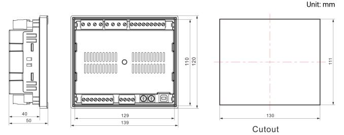
Fig. 12 - Installation Dimensions
