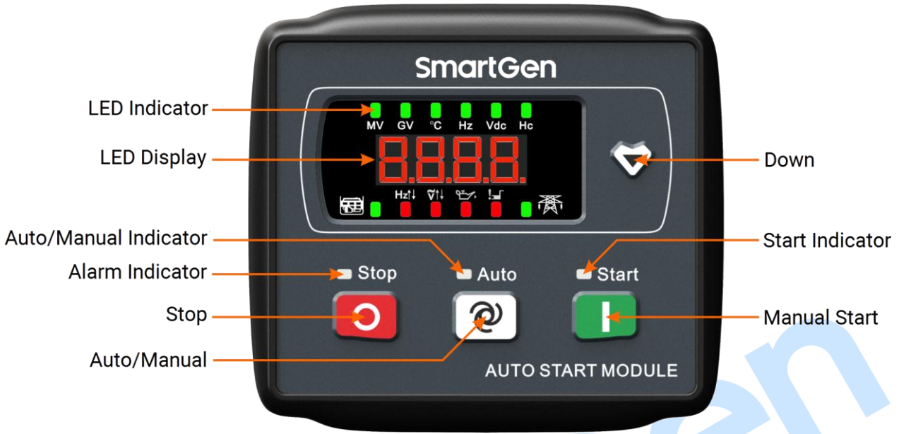
Fig.1 Front Panel Description
