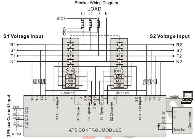
MCH: Stored Energy Motor; MN: Under Voltage Trip; MX: Open Relay; XF: Close Relay;
