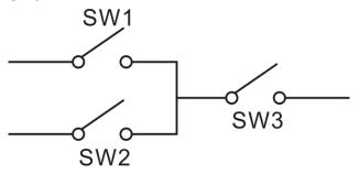
SW1 or SW2 is **TRUE**, while SW3 is **TRUE**, Defined combination output is active;
