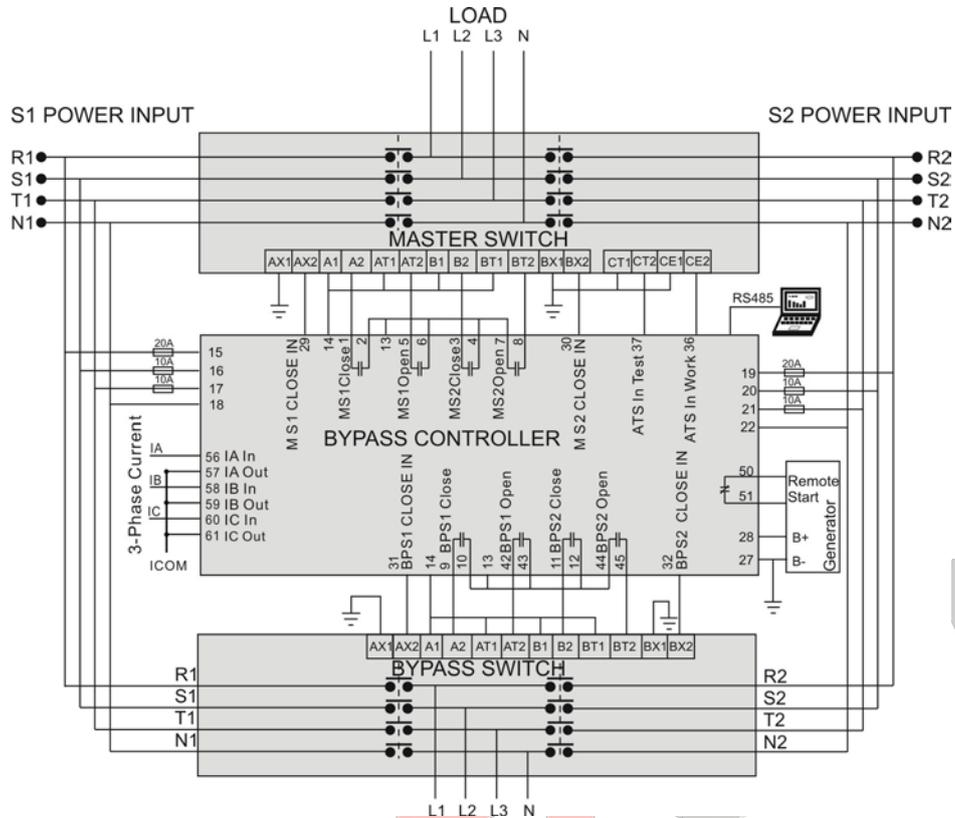
**Fig. 9 - Remote Control Application Diagram of Dual Bypass**
