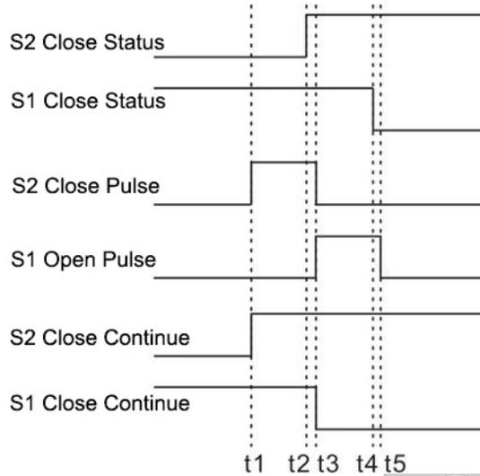
Fig. 5 - S2 Sync Close Procedure Oscillogram
