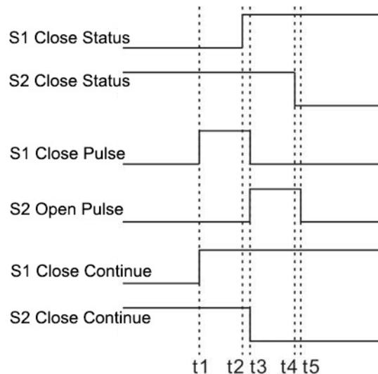
**Fig. 4 - S1 Sync Close Procedure Oscillogram**
