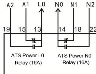
Fig. 6 - Internal Wiring of ATS Power LO-NO Output
