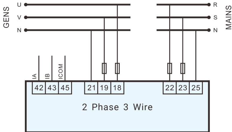
**Fig.6 – 2 Phase 3 Wire Diagram**
