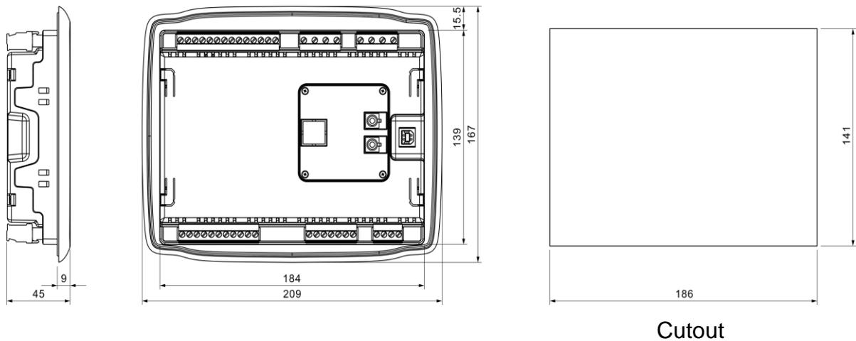
**Fig.8 – Case and Overall Dimensions (Unit: mm)**
