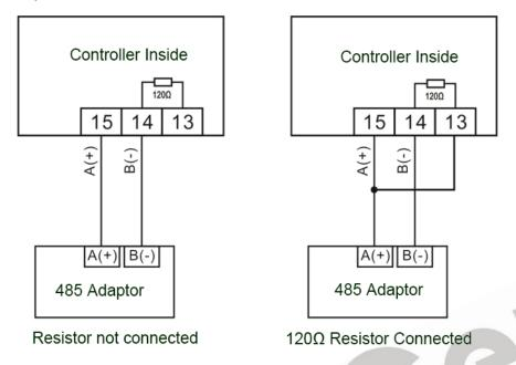
Fig. 7 - RS485 Connection Diagram
