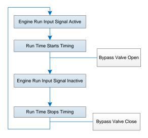
Fig. 3 - Engine Running Status Control Valve Open/Close Diagram
