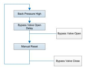
Fig. 4 - Back Pressure Control Valve Open Diagram
