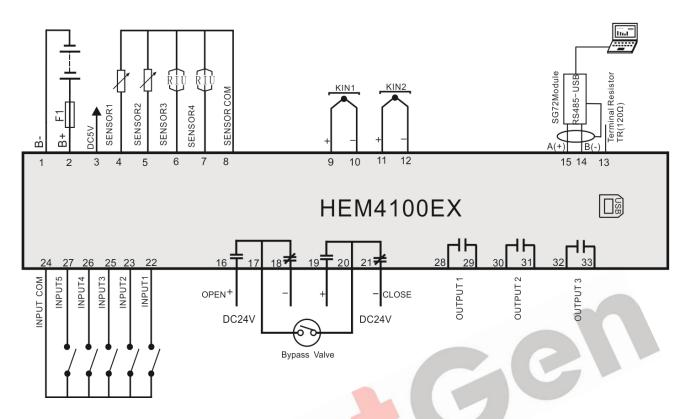
Fig. 8 - HEM4100EX Typical Application Diagram
