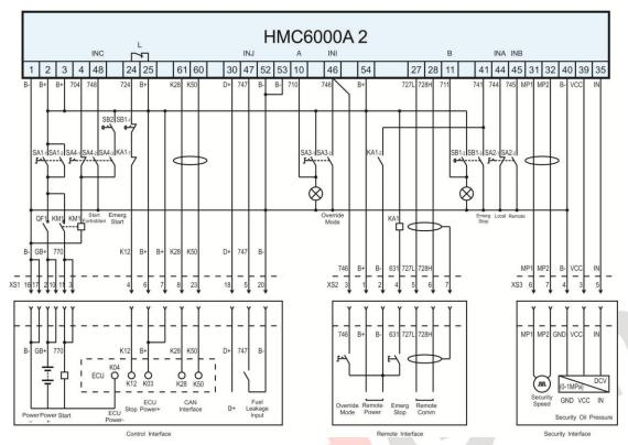
Figure 7: Control Box Wiring Diagram
