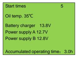
Figure 2: Measurement Data Display
