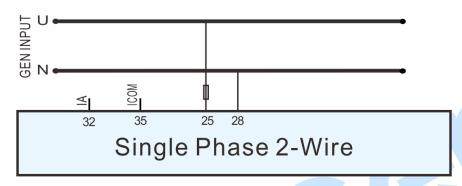
Fig.7 Single Phase 2-Wire Connection Diagram
