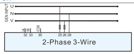
Fig. 6 2-Phase 3-Wire Connection Diagram
