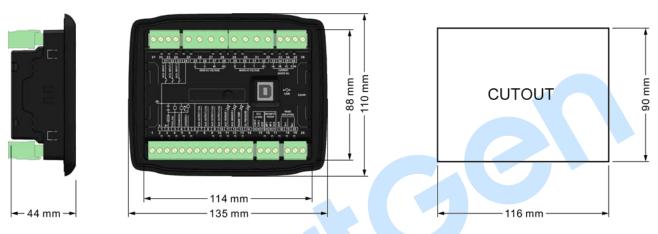
Fig.8 Overall Dimensions and Panel Cutout
