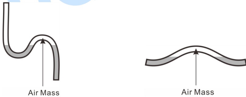
Fig.6 - Incorrect Pipe Connection Methods
