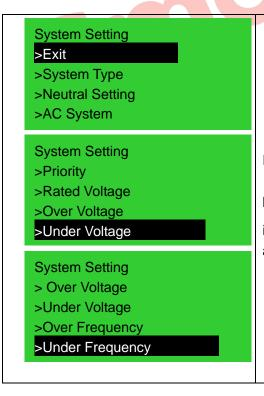
Press key to choose parameters (the current line was highlighted with black) and then press key to confirm, and it can enter into the corresponding display screen. Select >Exit and it will return to previous menu.
