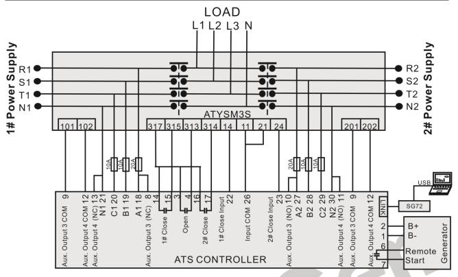
Fig. 10 ATYSM3S Wiring Diagram
