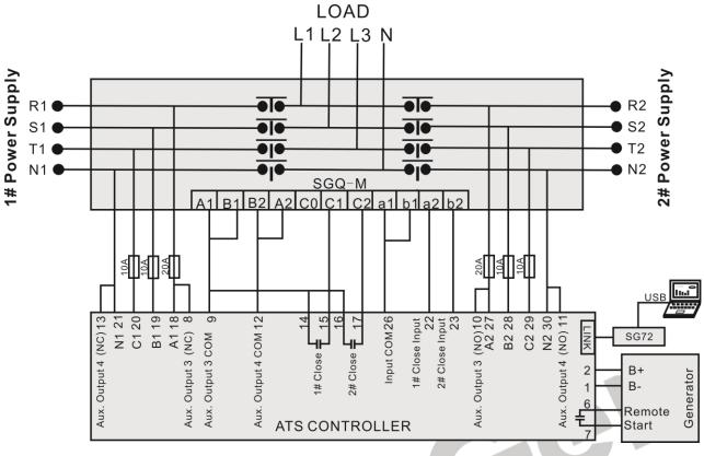
Fig. 6 SGQ-M Application Diagram
