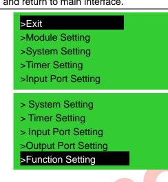
Press key to choose parameters (the current line was highlighted with black) and then press key to confirm, and it can enter into the corresponding display screen. Select >Exit and it will return to main display.
