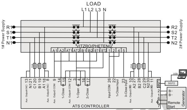
Fig. 8 VITZRO/PHETENG (Generator Start Control)
