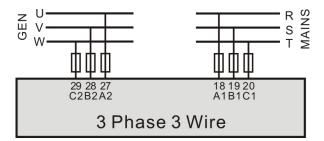
Fig. 12 3P3W Wiring Connection (take 1#Mains 2#Gens as an example)
