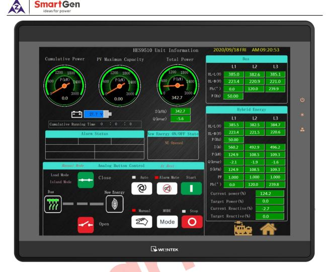
Fig.4 - HES9510 Genset Information of Controller Display
