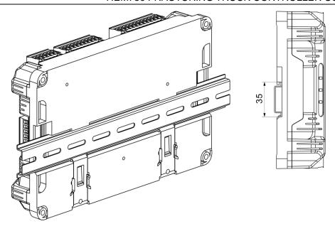
Fig.17-Guide Rail Installation
