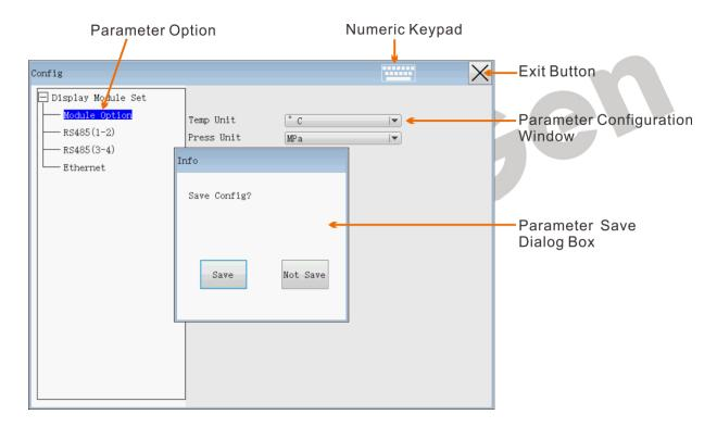
Fig.8-Parameter Configuration Interface of Display Module
