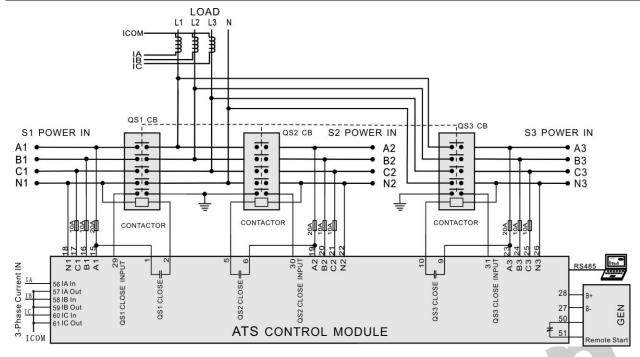
Fig.6 – Contactor Application Diagram
