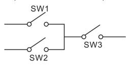
SW1 or SW2 is **TRUE**, while SW3 is **TRUE**, Defined combination output is active;
