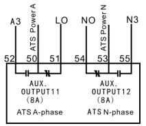
Fig.3 –Wring of ATS Supplied by Any of S1S2S3
