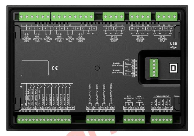
Fig.4 – Controller Rear Panel Drawing
