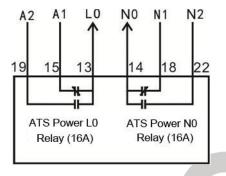
Fig.2 – Internal Wiring of ATS Power LO-NO Output
