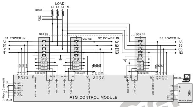
Fig.5 – Breaker Application Diagram
