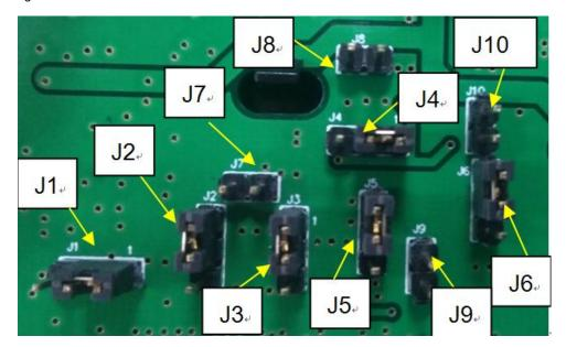
Fig.3 - Jumper Plug Transition Diagram
