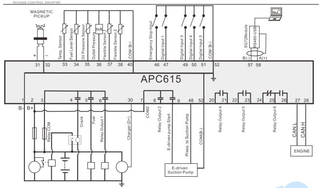
Fig. 7 - Typical Application with Electric Driven Suction Pump
