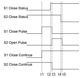
Fig. 4 - S1 Sync Close Procedure Oscillogram
