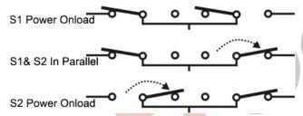
Fig. 3 - Sync Transfer Diagram
