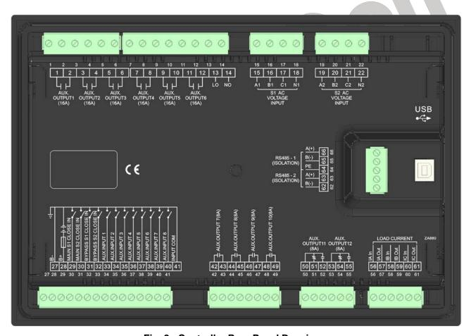
Fig. 8 - Controller Rear Panel Drawing
