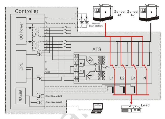
Note: The above drawing is suitable for N type and T type switch (SGQ), please refer to SGQ instruction for more details about M type switch.
