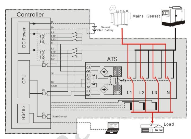
Note: The above drawing is suitable for N type and T type switch (SGQ), please refer to SGQ instruction for more details about M type switch.
