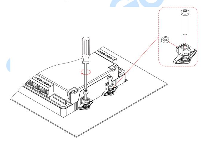
Fig.10 - Clips Installation Drawing
