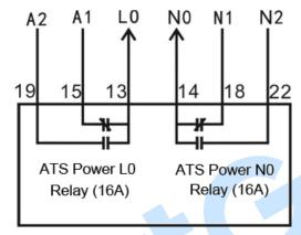
Fig.3 - Internal Wiring of ATS Power LO-NO Output
