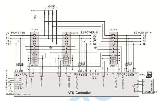
Fig.7 - Breaker Application Diagram
