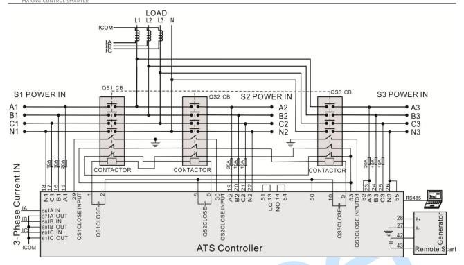
Fig.8 - Contactor Application Diagram
