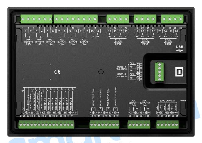
Fig.7 - Controller Rear Panel Drawing
