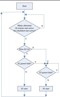
Fig.3 – Master Run Start Flow Diagram
