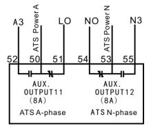
Fig.6 – Wring of ATS Supplied by Any of S1S2S3
