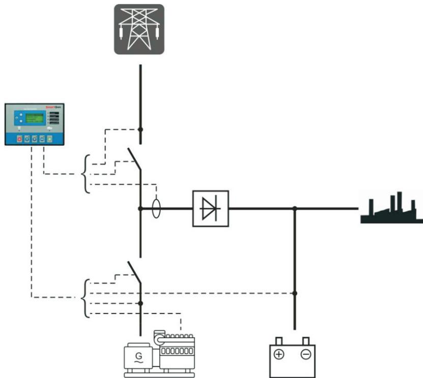
Control a different type of gensets, monitor temperature of generator room and voltage of storage battery, realize mains/load and mains/air-condition dual power automatic switch, and send short message when the genset alarm.
